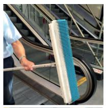
The REN Clean system's engineered pad removes soil from escalator treads without wear and tear."
